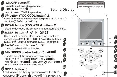
(\* Only for Heat Pump).FEEL mode can select the operation mode such as COOL,DRY,FAN,HEAT automatically depending on the room temperature,and the feel mode is default setting at starting.
